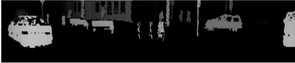
Filtered & interpolated Velodyne (i3D) range image
