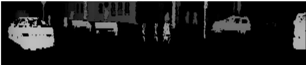
Filtered & interpolated Velodyne (i3D) range image
